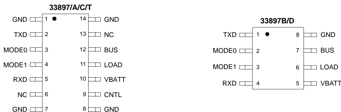
Figure 4. 33897/A/B/C/D/T Pin Connections
