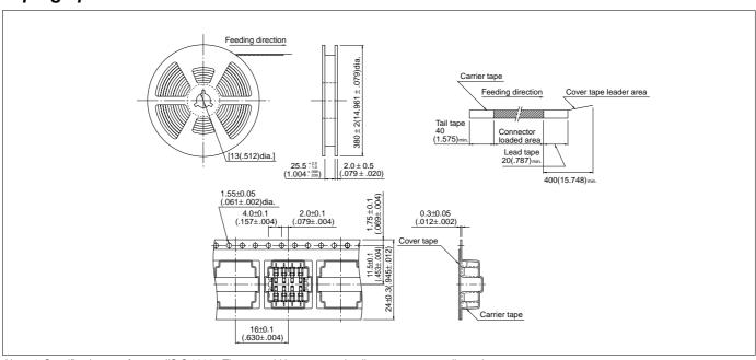
Note: 1. Specifications conform to JIS C 0806. The tape width, connector loading recess square dimensions, etc.are determined by the number of circuits and external shape of the connector to be loaded.
