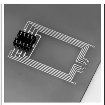
The ICC connector is designed to be accommodated within IC card reading/writing devices. The market for IC cards is rapidly expanding and replacing magnetic cards. The ICC connector is compatible with IC cards which conform to ISO7816.
