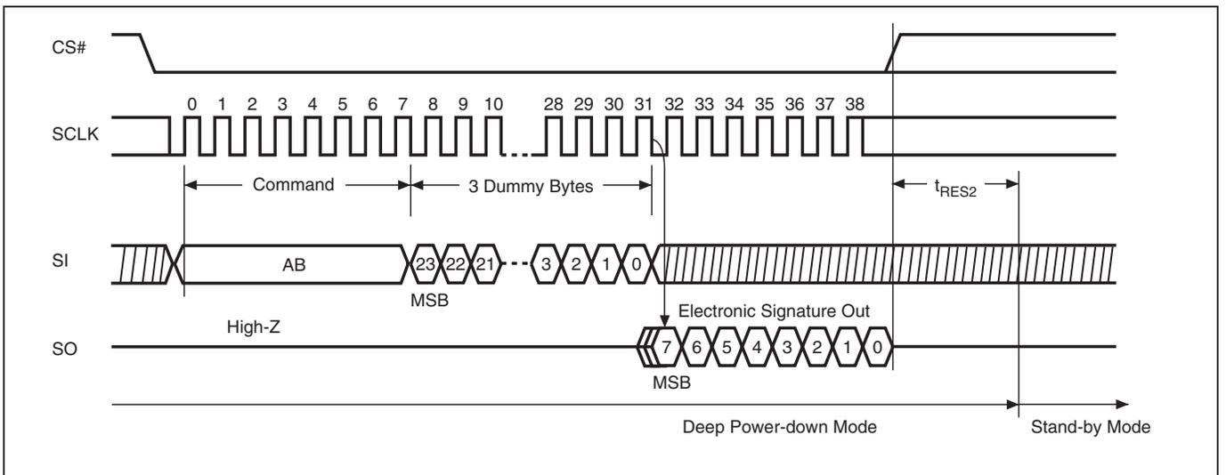
**Figure 24. Release from Deep Power-down (RDP) Sequence (Command AB)**
