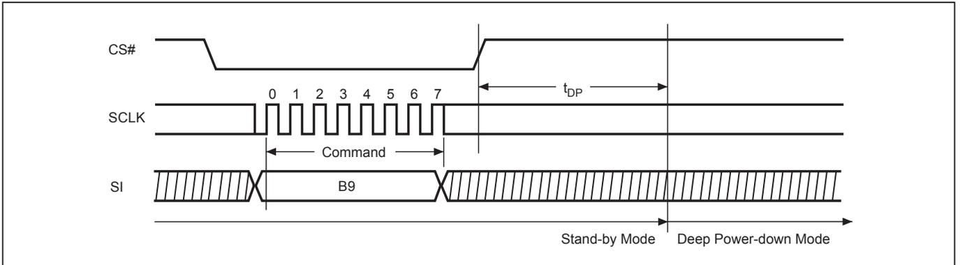
**Figure 23. Release from Deep Power-down and Read Electronic Signature (RES) Sequence (Command AB)**
