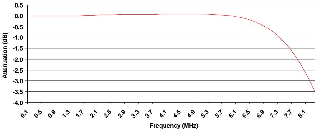
Figure 4. FMS6646 SD Frequency Response (Flatness)
