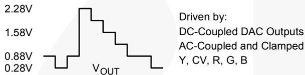
There is a 280mV offset from the DC input level to the DC output level.  $V_{OUT} = 2 \cdot V_{IN} + 280mV$ .
