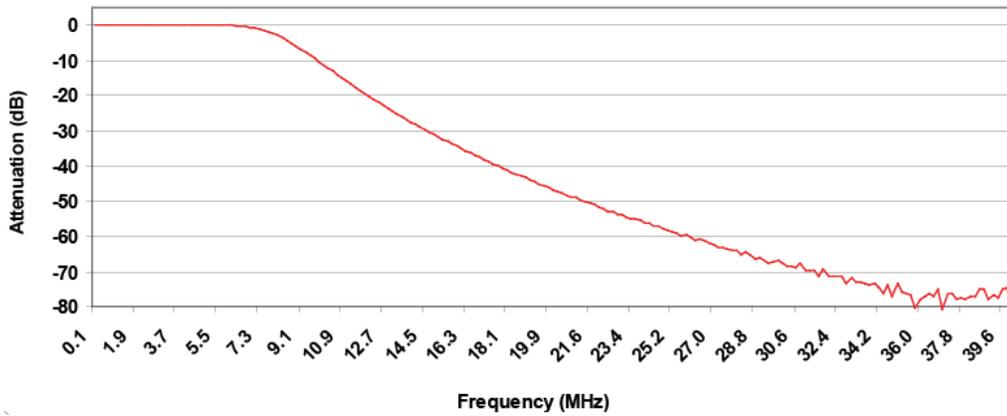
Figure 3. FMS6646 SD Frequency Response
