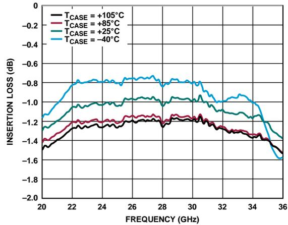
Figure 8. Insertion Loss vs. Frequency, RF1 Selected
