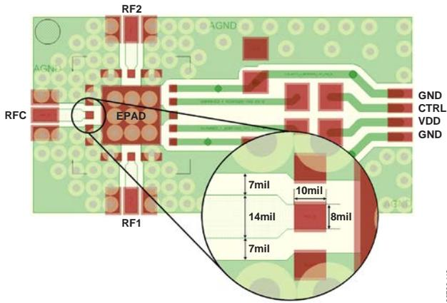
Figure 18. Probe Matrix Board, Top Layer
