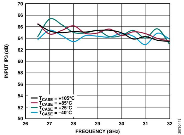
Figure 13. Input IP3 vs. Frequency, RF2 Selected
