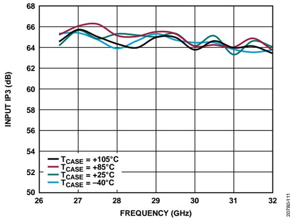
Figure 11. Input IP3 vs. Frequency, RF1 Selected
