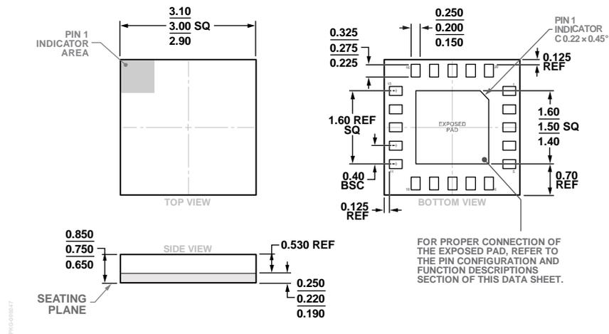
Figure 19. 20-Terminal Land Grid Array [LGA]
