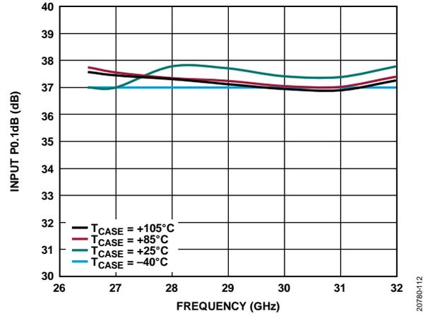
Figure 12. Input P0.1dB vs. Frequency, RF2 Selected
