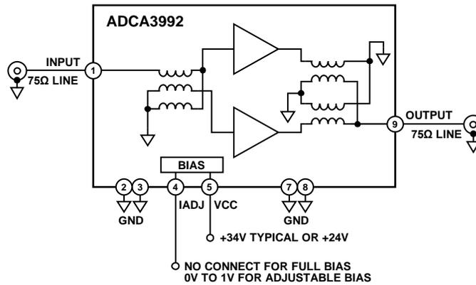
Figure 11. Basic Connections
