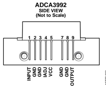
Figure 2. Pin Configuration
