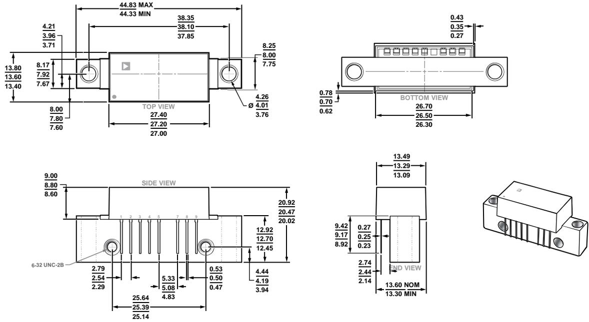
Figure 12. 8-Pin SOT115J Module Package [MODULE] (ML-8-1)
