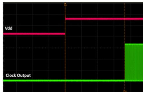
**Figure 16. Startup Waveform vs. Vdd**
