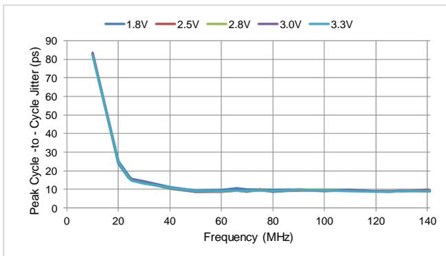
Figure 12. Cycle-to-cycle Jitter vs Frequency
