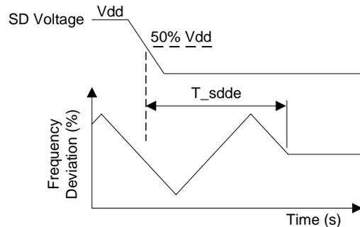
Figure 7. SD Diable Timing (SD Mode Only)
