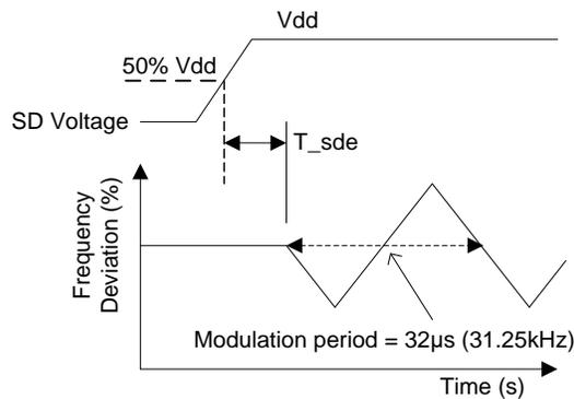
Figure 6. SD Enable Timing (SD Mode Only)
