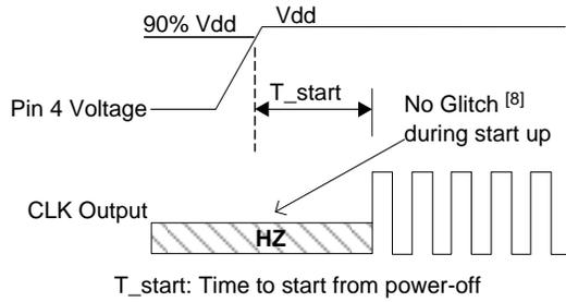
Figure 2. Startup Timing
