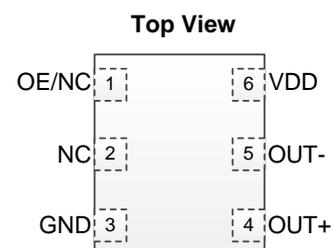
**Figure 3. Pin Assignments**
