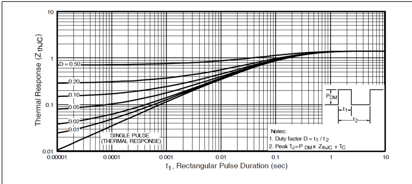
**Figure 4 Maximum Thermal Impedance  $Z_{thJC}$  Characteristics (Per Leg)**
