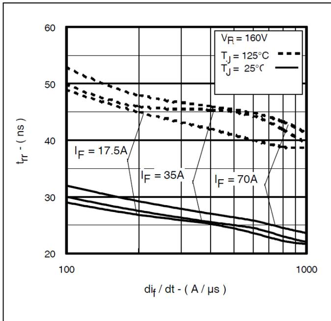
**Figure 5 Typical Reverse Recovery Vs.  $di/dt$  (Per Leg)**
