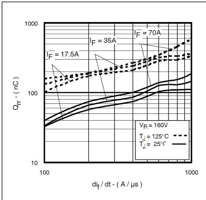
**Figure 7 Typical Stored Charge Vs. dif/dt (Per Leg)**
