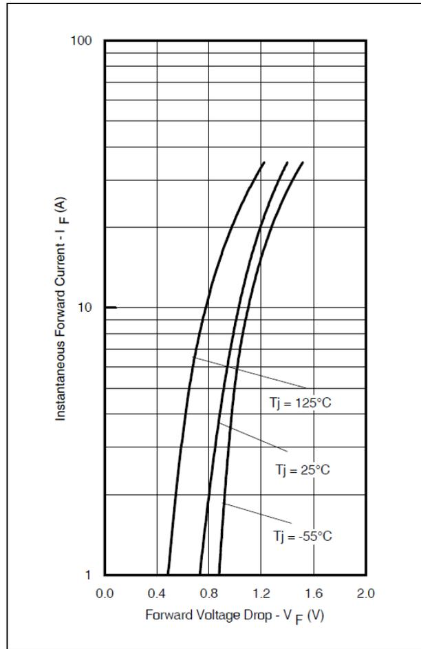
**Figure 1 Maximum Forward Voltage Drop Characteristics (Per Leg)**
