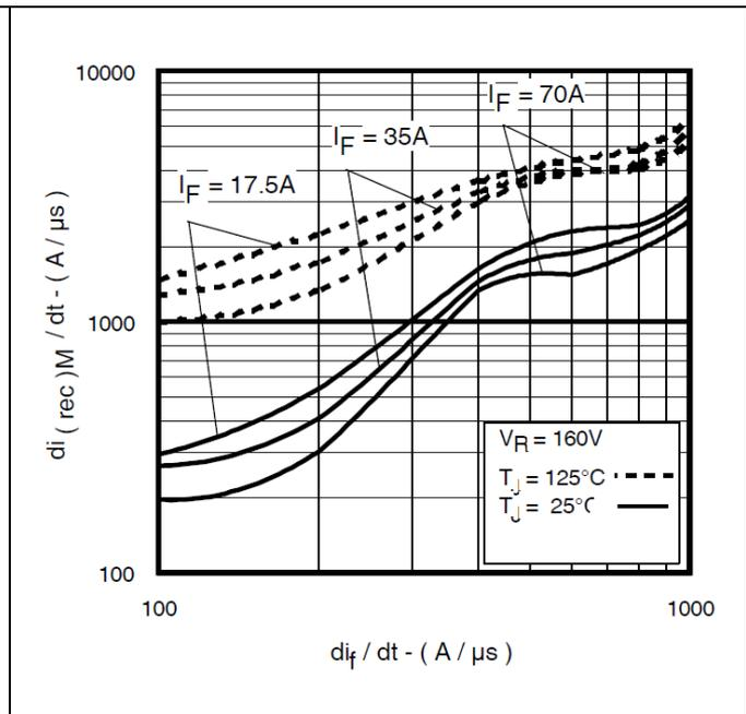
**Figure 8 Typical di(rec)M/dt Vs. dif/dt (Per Leg)**
