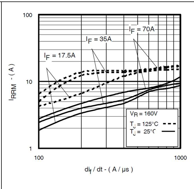
**Figure 6 Typical Recovery Current Vs.  $di/dt$  (Per Leg)**
