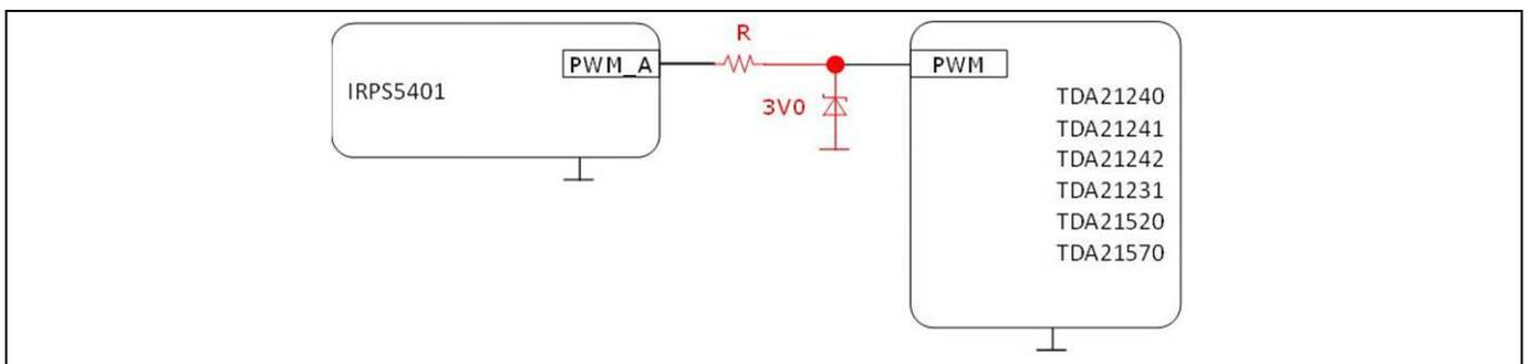
**Figure 11 Zener clamp details when using power stages that only support 3.3V PWM input**
