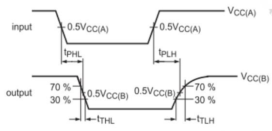
**Figure 6: Propagation Delay and Transition Times A→B**
