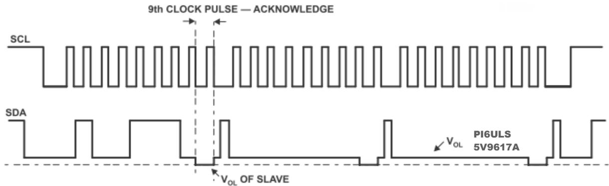
Figure 13: Bus B (2.2V to 5.5V Bus) Waveform
