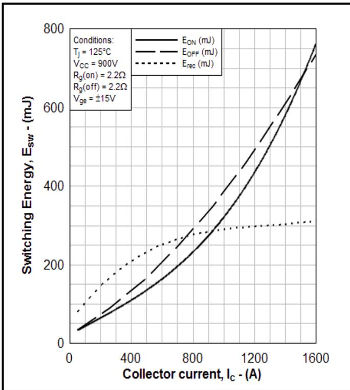
Fig. 5 Typical switching energy vs collector current
