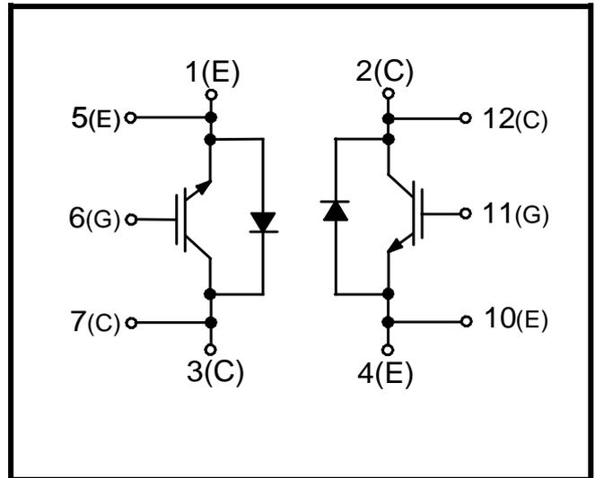
**Fig. 1 Circuit configuration**
