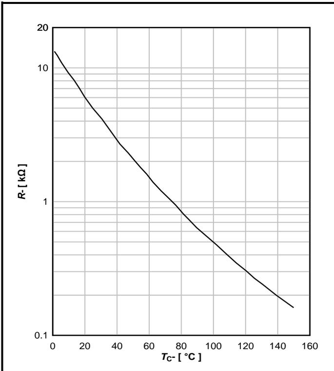
Fig. 9 Typical NTC thermistor characteristics
