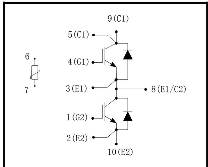
**Fig. 1 Circuit configuration**
