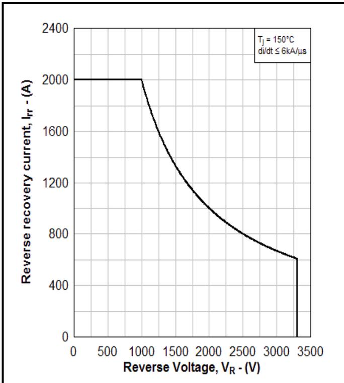
Fig. 9 Diode reverse bias safe operating area
