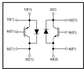
Fig. 1 Circuit configuration
