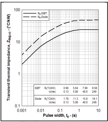
Fig. 10 Transient thermal impedance
