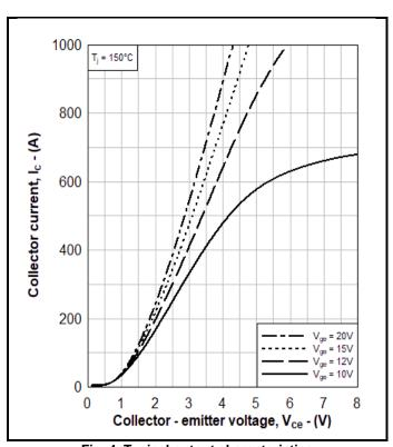
Fig. 4 Typical output characteristics
