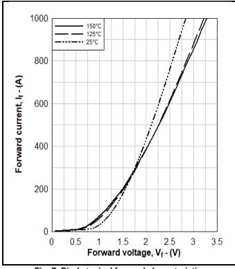
Fig. 7 Diode typical forward characteristics
