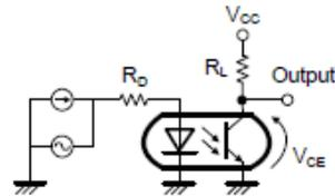
**Fig.17 Test Circuit for Common Mode Rejection Voltage**
