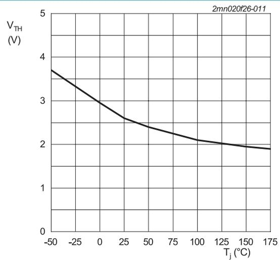
$V_{DS} = 10\text{ V}$ ;  $I_{DS} = 20\text{ mA}$
