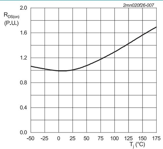
$I_{DS} = 50\text{ A}; V_{GS} = 18\text{ V}; t_p < 200\ \mu\text{s}$
