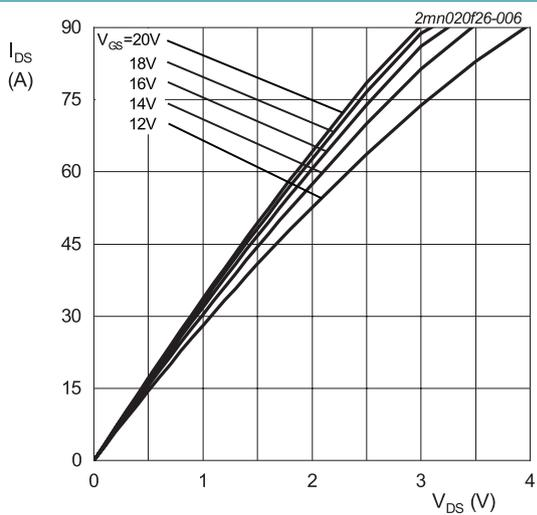
$T_j = 175\text{ °C}; t_p < 200\ \mu\text{s}$
