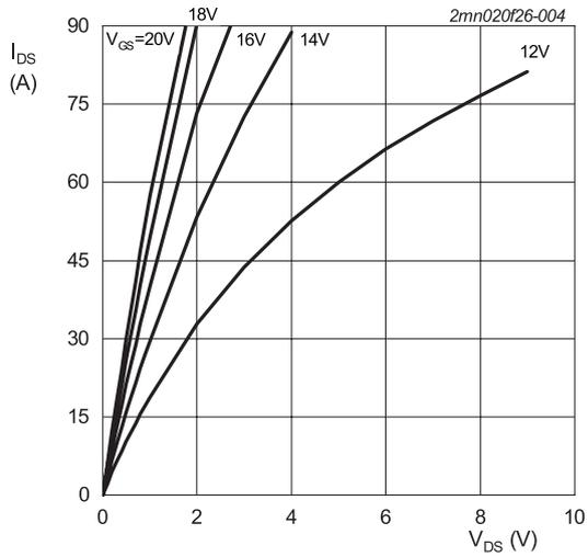
$T_j = -55\text{ °C}; t_p < 200\ \mu\text{s}$
