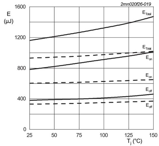
$I_{DS} = 50\text{ A}$ ;  $V_{DD} = 800\text{ V}$ ;  $R_{G(ext)} = 2.4\ \Omega$ ;
