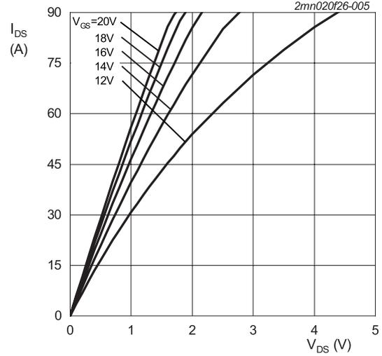
$T_j = 25\text{ °C}; t_p < 200\ \mu\text{s}$
