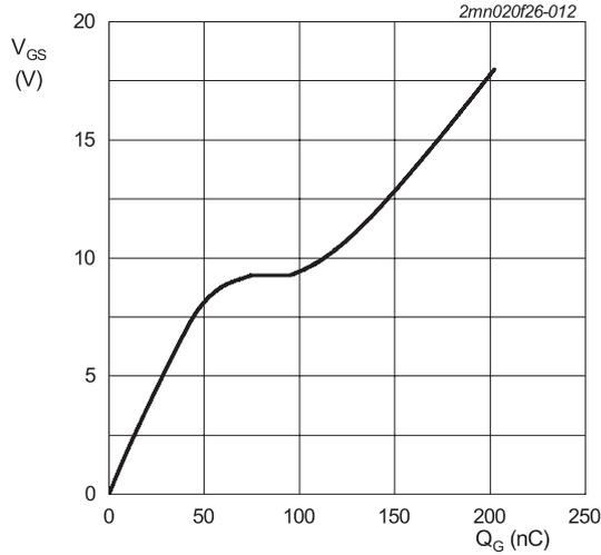
$I_{DS} = 50 \text{ A}; I_{GS} = 0.1 \text{ mA}; V_{DS} = 800 \text{ V}; T_j = 25 \text{ }^\circ\text{C}$
