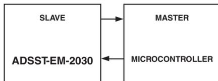
Figure 1. SPI Communication between ADSST-EM-2030 and Microcontroller
