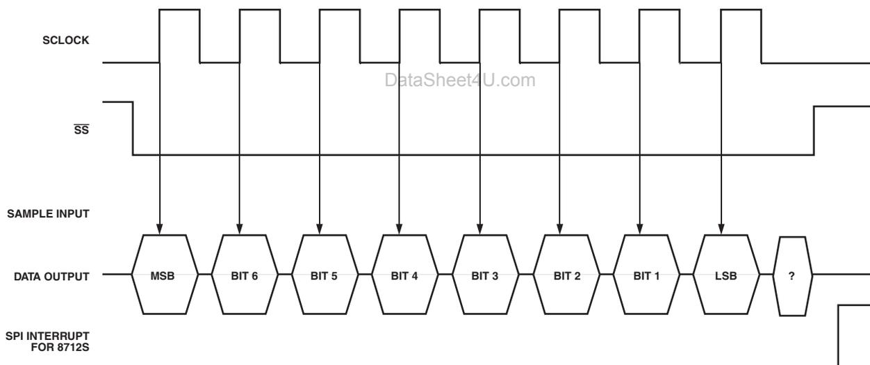
Figure 3. SPI Timing for Data Transmission Byte
