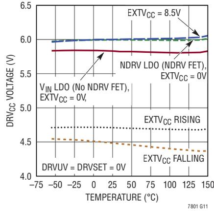
**EXT<sub>V<sub>CC</sub></sub> Switchover and DRV<sub>CC</sub> Voltages vs Temperature**
