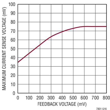
**Maximum Current Sense Threshold vs I<sub>TH</sub> Voltage**
