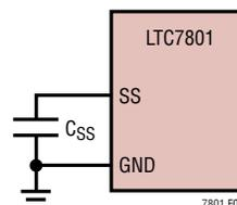
Figure 6. Using the SS Pin to Program Soft-Start
