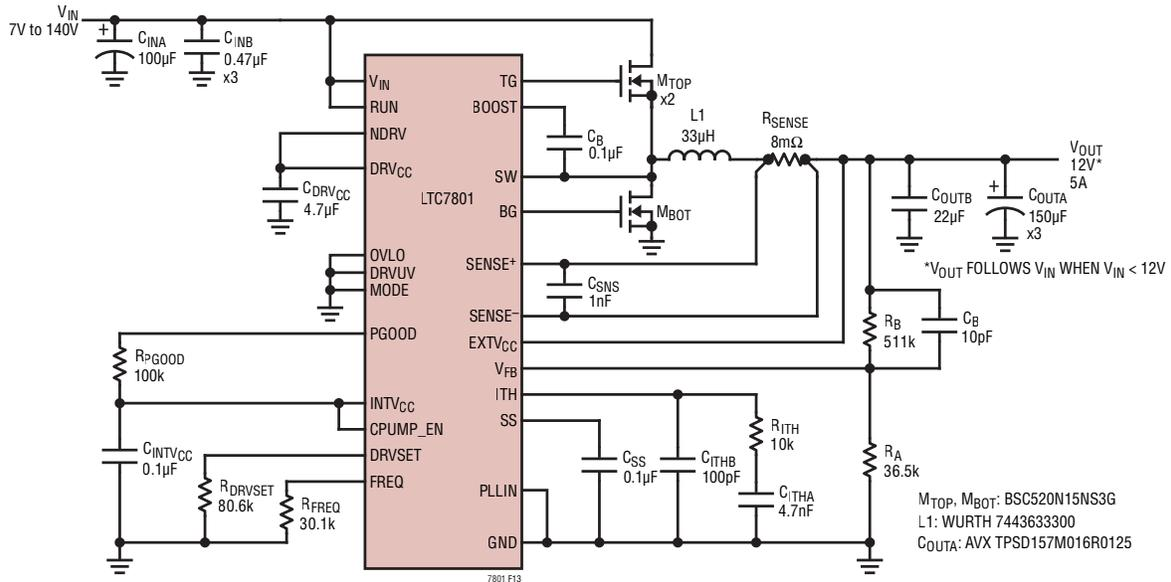
Figure 13. High Efficiency 140V to 12V Step-Down Regulator
