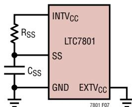
**Figure 7. Using the SS Pin to Program Soft-Start with EXTV<sub>CC</sub> Unused/Grounded to Defeat REGSD**
