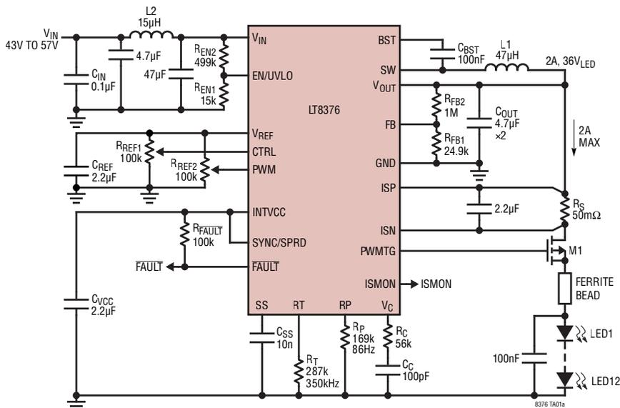
Internal PWM Dimming
