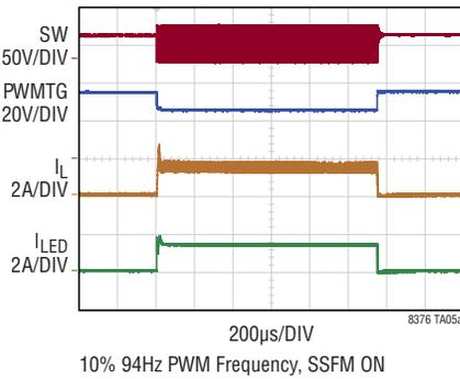
Internal PWM Dimming
