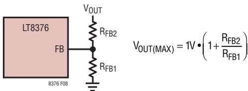
Figure 8. Resistor Configuration
