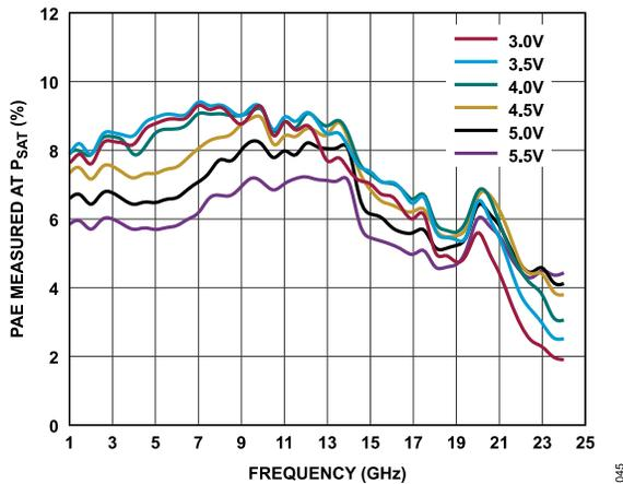
Figure 45. PAE Measured at  $P_{SAT}$  vs. Frequency for Various Supply Voltages, 1 GHz to 24 GHz,  $I_{DQ} = 110$  mA
