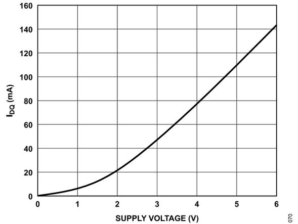
Figure 70.  $I_{DQ}$  vs. Supply Voltage,  $R_{BIAS} = 1150\ \Omega$
