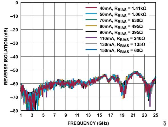
Figure 28. Reverse Isolation vs. Frequency for Various  $I_{DQ}$  and  $R_{BIAS}$  Values, 1 GHz to 25 GHz,  $V_{DD} = 3 V$
