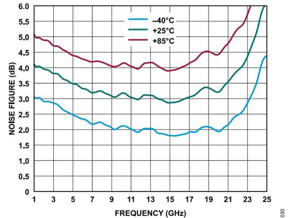
Figure 30. Noise Figure vs. Frequency for Various Temperatures, 1GHz to 25 GHz,  $V_{DD} = 3 V$ ,  $I_{DQ} = 47 mA$ ,  $R_{BIAS} = 1150 \Omega$
