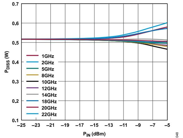
Figure 48.  $P_{DISS}$  vs.  $P_{IN}$  at Various Frequencies,  $T_{CASE} = 85^\circ\text{C}$ ,  $V_{DD} = 5$  V
