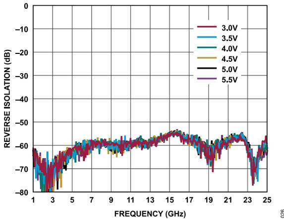
Figure 26. Reverse Isolation vs. Frequency for Various Supply Voltages, 1 GHz to 25 GHz,  $I_{DQ} = 110 mA$
