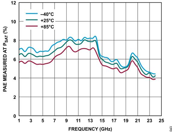
Figure 43. PAE Measured at  $P_{SAT}$  vs. Frequency for Various Temperatures, 1 GHz to 24 GHz,  $V_{DD} = 5$  V,  $I_{DQ} = 110$  mA,  $R_{BIAS} = 1150 \Omega$
