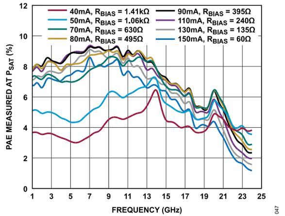
Figure 47. PAE Measured at  $P_{SAT}$  vs. Frequency for Various  $I_{DQ}$  and  $R_{BIAS}$  Values, 1 GHz to 24 GHz,  $V_{DD} = 3$  V
