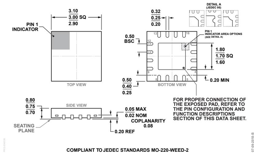
**Figure 79. 16-Lead Lead Frame Chip-Scale Package [LF CSP]
