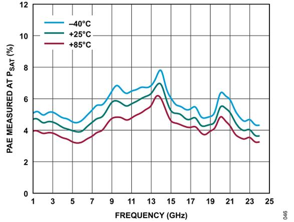
Figure 46. PAE Measured at  $P_{SAT}$  vs. Frequency for Various Temperatures, 1 GHz to 24 GHz,  $V_{DD} = 3$  V,  $I_{DQ} = 47$  mA,  $R_{BIAS} = 1150 \Omega$
