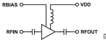
Figure 74. Simplified Schematic
