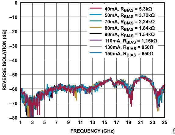
Figure 25. Reverse Isolation vs. Frequency for Various  $I_{DQ}$  and  $R_{BIAS}$  Values, 1 GHz to 25 GHz,  $V_{DD} = 5 V$
