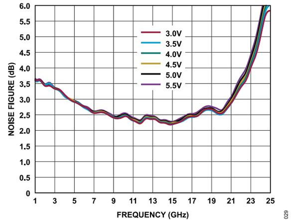
Figure 29. Noise Figure vs. Frequency for Various Supply Voltages, 1 GHz to 25 GHz,  $I_{DQ} = 110 mA$
