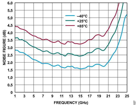
Figure 27. Noise Figure vs. Frequency for Various Temperatures, 1 GHz to 25 GHz,  $V_{DD} = 5 V$ ,  $I_{DQ} = 110 mA$ ,  $R_{BIAS} = 1150 \Omega$
