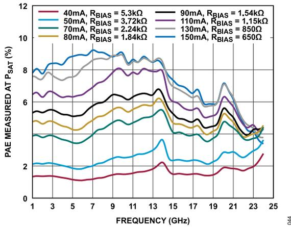
Figure 44. PAE Measured at  $P_{SAT}$  vs. Frequency for Various  $I_{DQ}$  and  $R_{BIAS}$  Values, 1 GHz to 24 GHz,  $V_{DD} = 5$  V
