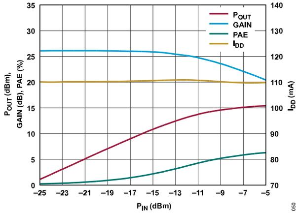
Figure 50.  $P_{OUT}$ , Gain, PAE, and  $I_{DD}$  vs.  $P_{IN}$ , Power Compression at 5 GHz,  $V_{DD} = 5 V$ ,  $R_{BIAS} = 1150 \Omega$
