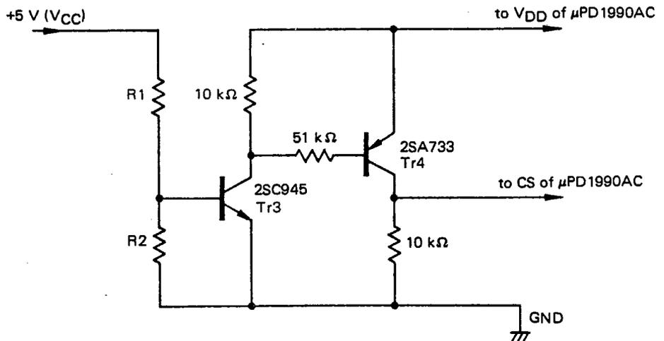
The Power Down of  $V_{CC}$  line makes CS terminal inactive, with R1 and R2 resistors. The trigger level of this circuit is calculated as following.
