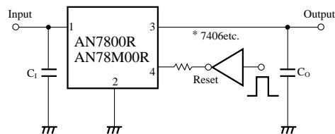
\* For TTL, an open collector type inverter, buffer, gate etc. can be used.
