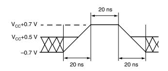
Figure 9. Maximum Positive Overshoot Waveform
