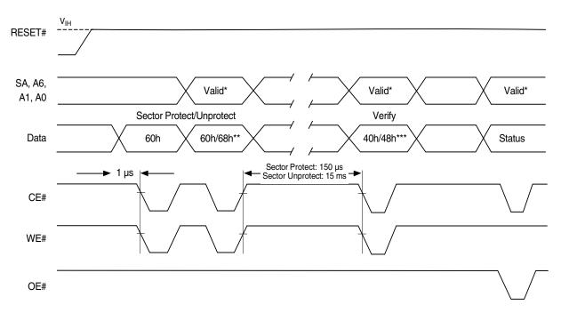
\* Valid address for sector protect: A6 = 0, A1 = 1, A0 = 0. Valid address for sector unprotect: A6 = 1, A1 = 1, A0 = 0.
