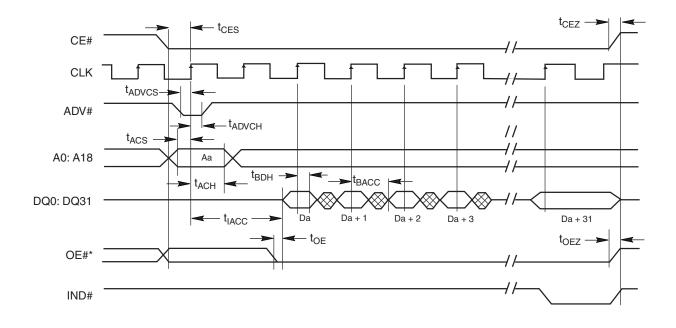
Figure 16. Burst Mode Read (x32 Mode)
