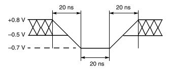
Figure 8. Maximum Negative Overshoot Waveform
