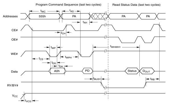
**Note:** PA = program address, PD = program data,  $D_{OUT}$  is the true data at the program address.
