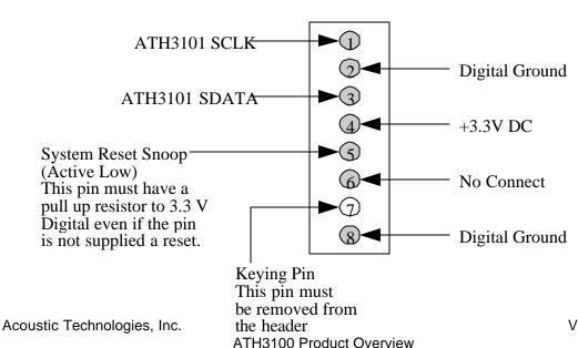
Figure 4: SIB-232 Dongle Header Pin Out
