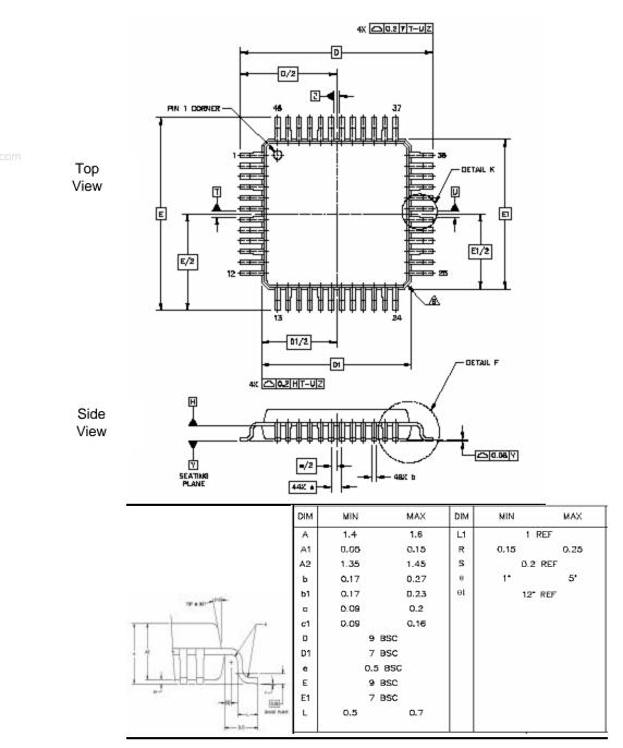
Figure 2: ATH3100 48-Pin LQFP Package Outline Diagram (dimensions are in millimeters)
