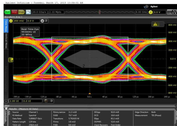
Figure 81. Eye at 5-Gbps Bit Rate with Increased Output Swing
