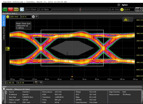
Figure 86. Eye at 5-Gbps Bit Rate with Default Output Swing
