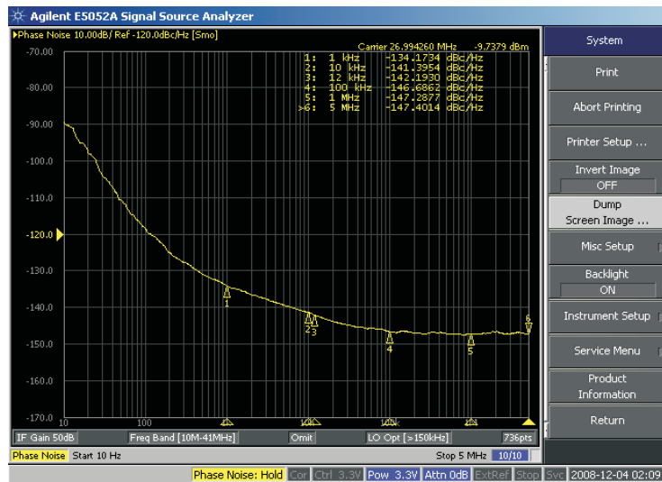
Figure 2. Phase Noise Plot, x1 Mode, 0% SSC, 27 MHz Crystal
