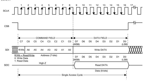
Figure 15. Serial Interface Protocol
