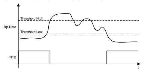
Figure 11. Behavior Of INTB Terminal In Comparator Mode
