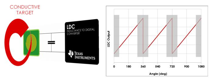
Figure 21. Angular Position Sensing
