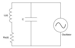
Figure 7. LC Tank Connected To Oscillator
