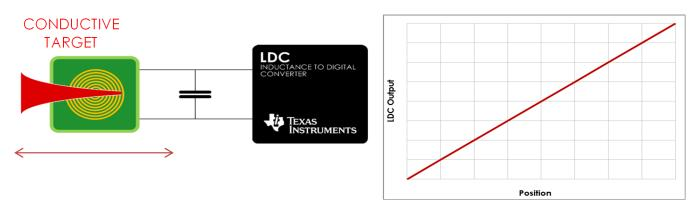
Figure 20. Linear Position Sensing
