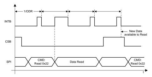
Figure 13. Behavior of INTB Terminal in DRDYB Mode with SPI Extending Beyond Subsequent Conversions
