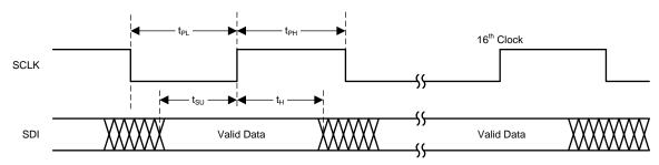
Figure 1. Write Timing Diagram
