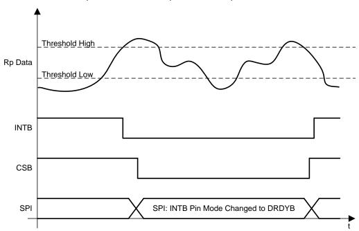
Figure 12. Behavior Of INTB Terminal In Wake-Up Mode
