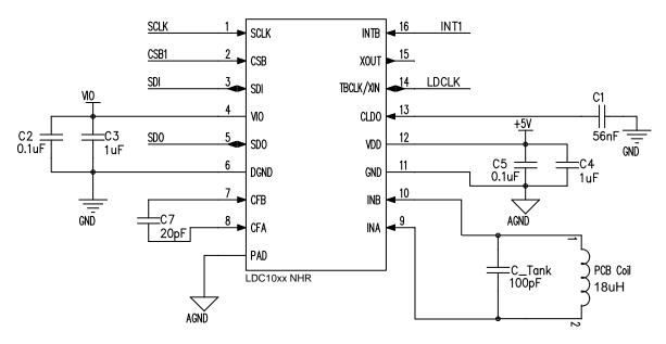
Figure 16. Typical Application Schematic, LDC10xx
