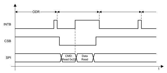
Figure 14. Behavior Of INTB Terminal In DRDYB Mode with SPI Reading The Data Within Subsequent Conversion
