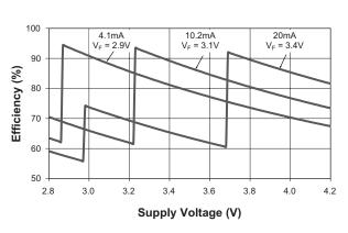
Efficiency vs. Supply Voltage
