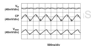
Load Characteristics (V<sub>IN</sub> = 3.1V; 2X Mode; 20mA Load)
