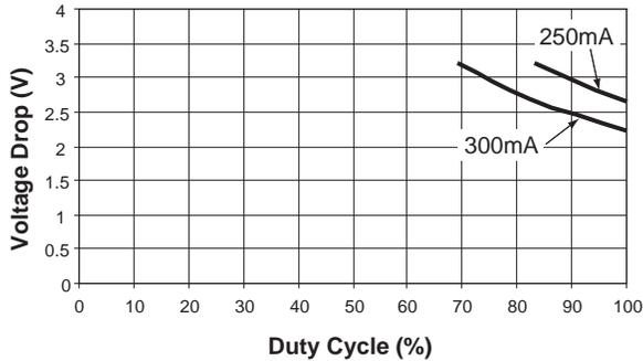
**Device Duty Cycle vs.  $V_{DROD}$**
