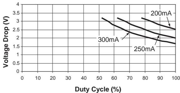
**Device Duty Cycle vs.  $V_{DROD}$**
