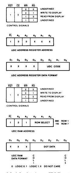
Figure 3. Logic Levels to Access a UDC Character.
