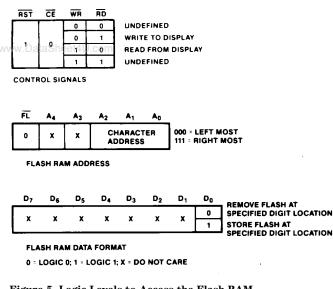
Figure 5. Logic Levels to Access the Flash RAM.
