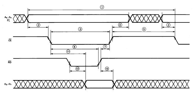
INPUT PULSE LEVELS: 0.6 V TO 2.4 V OUTPUT REFERENCE LEVELS: 0.6 V TO 2.2 V OUTPUT LOADING = 1 TTL LOAD AND 100pF
