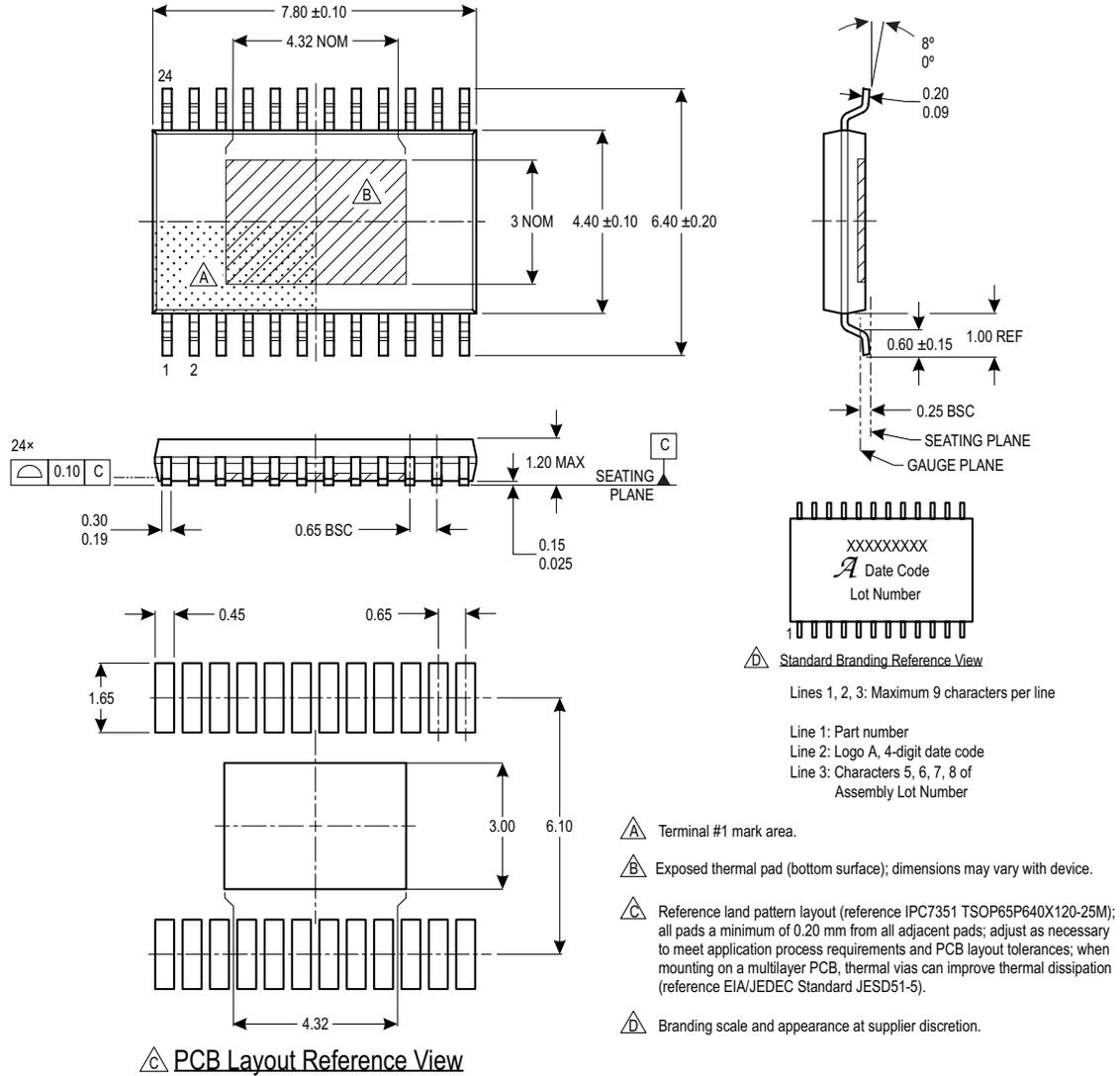
Figure 11: Package LP, 24-Lead TSSOP with Exposed Pad
