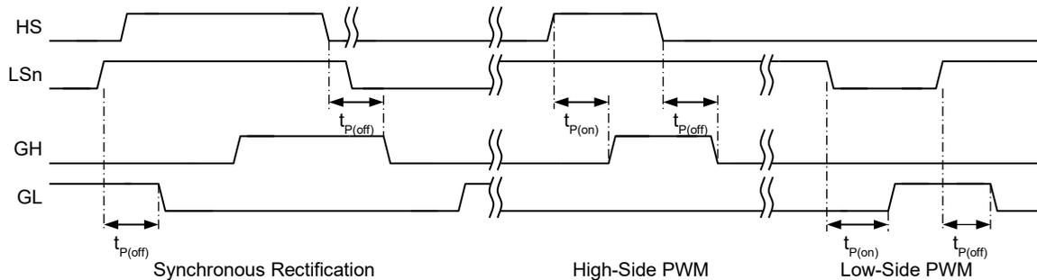
Figure 5: Gate Drive Timing – Control Inputs
