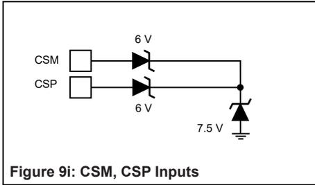
Figure 9i: CSM, CSP Inputs
