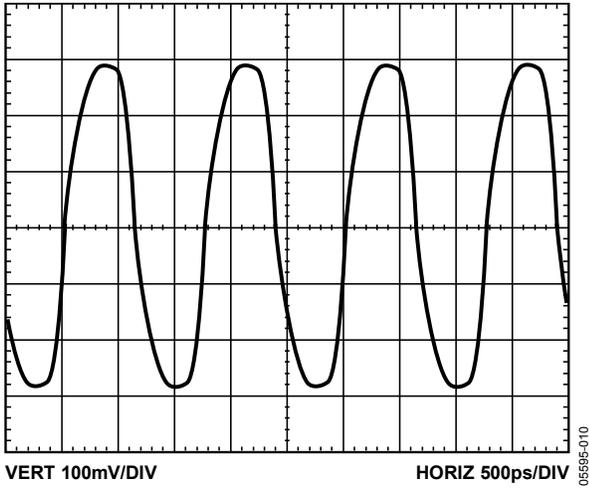
Figure 9. LVDS Differential Output at 800 MHz
