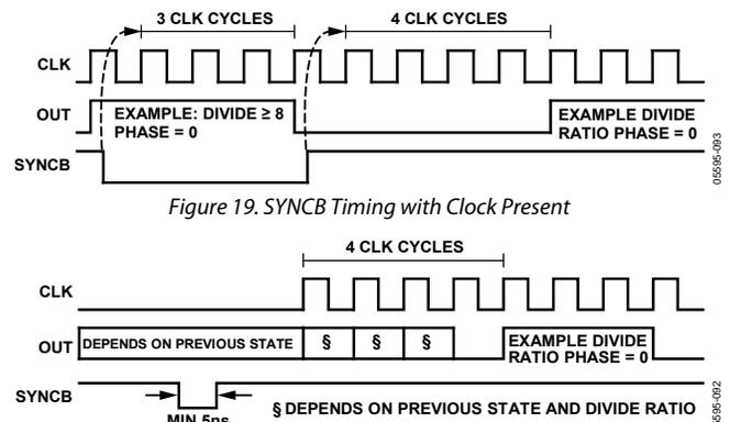
Figure 20. SYNCB Timing with No Clock Present
