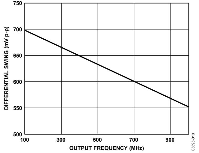
Figure 11. LVDS Differential Output Swing vs. Frequency
