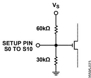
Figure 22. Setup Pin ( $S_0$  to  $S_{10}$ ) Equivalent Circuit
