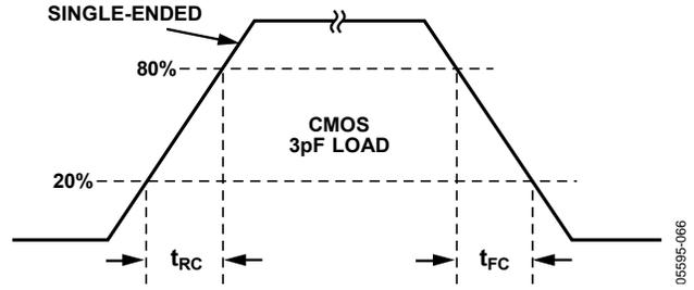
Figure 4. CMOS Timing, Single-Ended, 3 pF Load
