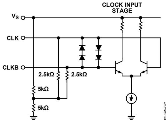
Figure 17. Clock Input Equivalent Circuit
