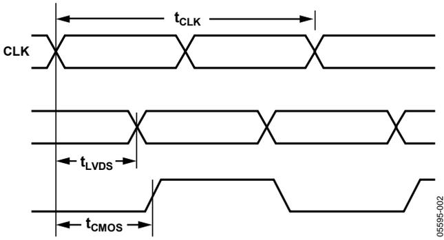
Figure 2. CLK/CLKB to Clock Output Timing, DIV = 1 Mode
