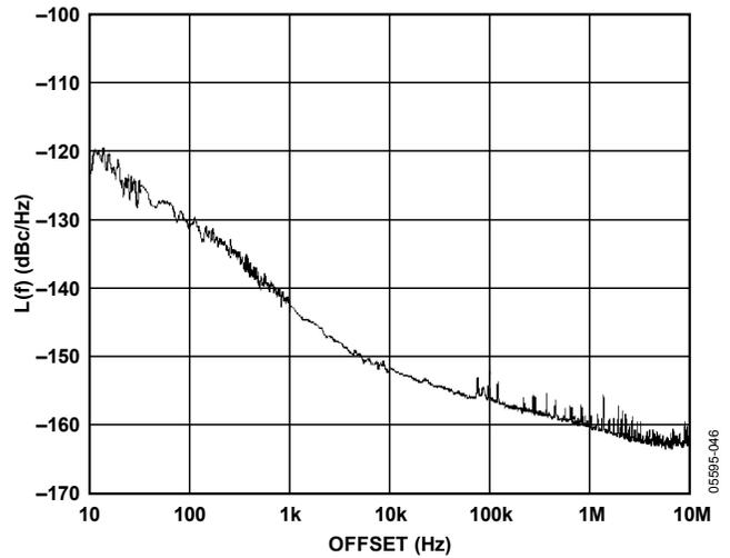
Figure 16. Additive Phase Noise—CMOS DIV4, 61.44 MHz
