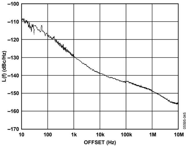
Figure 14. Additive Phase Noise—CMOS DIV 1, 245.76 MHz
