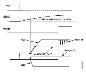
Figure 22. Power-Up Sequence Timing Diagram
