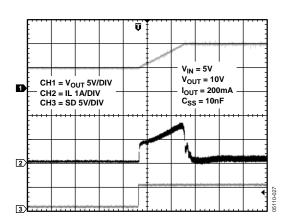
Figure 5. Start-Up Response from Shutdown, Css = 10 F
