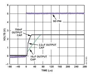
Figure 9. LDO Power-Up Response from Shutdown
