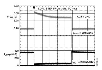
Figure 12. LDO Load Transient Response,  $V_{OUT} = 3.3 \text{ V}$
