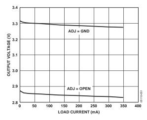
Figure 7. LDO Output Voltage vs. Load Current, VIN = 5 V
