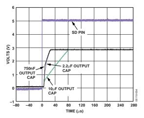
Figure 10. LDO Power-Up Response from Shutdown
