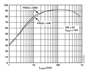
Figure 3. Efficiency vs. Load Current (mA)
