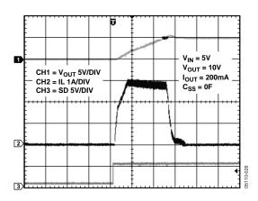
Figure 4. Start-Up Response from Shutdown,  $C_{SS} = 0 F$
