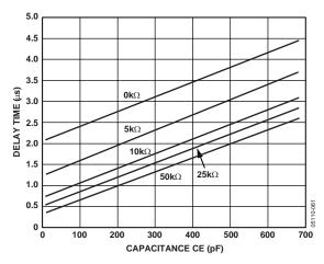
Figure 17. GPM Delay Time vs. CE Capacitance
