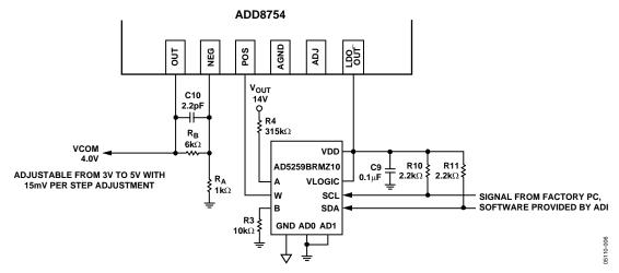
Figure 27. ADD8754 with Programmable V<sub>COM</sub>
