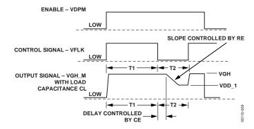
Figure 21. Gate Pulse Modulator Timing Diagram
