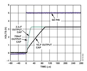
Figure 8. LDO Power-Up Response from Shutdown
