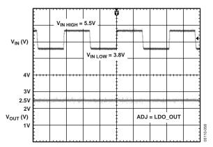
Figure 14. LDO Line Transient Response,  $V_{OUT} = 2.5 \text{ V}$
