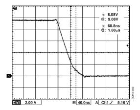
Figure 16.  $V_{COM}$  Falling Slew Rate,  $VDD_2 = 14 V$
