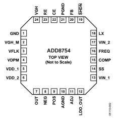
Figure 2. Pin Configuration
