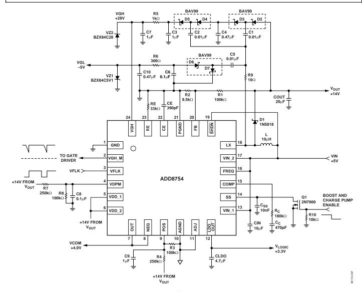
$\textit{Figure 26.} \ 1.2 \ \textit{MHz} \ \textit{Application Circuit for TFT LCD Display with LDO\_ALWAYS\_ON}$
