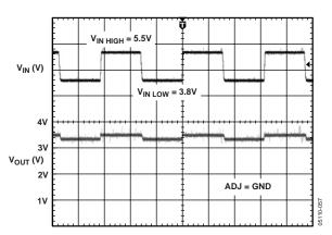
Figure 13. LDO Line Transient Response,  $V_{OUT} = 3.3 \text{ V}$
