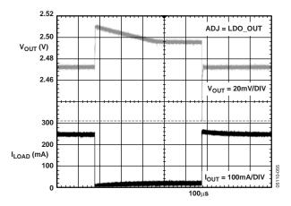
Figure 11. LDO Load Transient Response,  $V_{OUT} = 2.5 \text{ V}$
