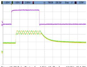
Figure 19. EN Pulse Timing,  $f_{IN} = 1$  GHz, 10 dBm,  $f_{OUT} = 10$  MHz, Ch3: EN, Ch2/1: IF Out
