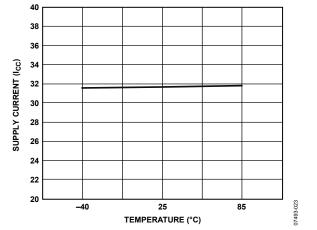
Figure 18. Supply Current (Icc) vs. Temperature with ALS Asserted, IIBIAS = 11 mA
