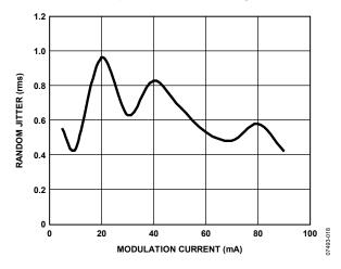
Figure 13. Random Jitter vs. Modulation Current,  $I_{IBIAS} = 20 \text{ mA}$
