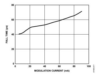
Figure 12. Fall Time vs. Modulation Current, I<sub>IBIAS</sub> = 20 mA
