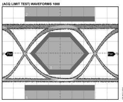
Figure 25. Optical Eye 155 Mbps, 1.078 ns/DIV, PRBS 2<sup>31-1</sup> P<sub>AV</sub> = -4.5 dBm, ER = 9 dB, Mask Margin 50%
