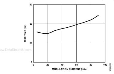
Figure 11. Rise Time vs. Modulation Current, IIBIAS = 20 mA
