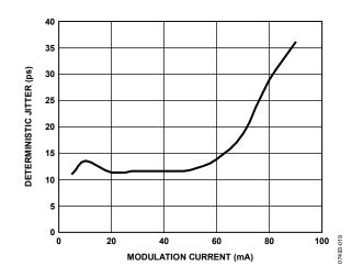
Figure 14. Deterministic Jitter at 4.25 Gbps vs. Modulation Current, I<sub>IBIAS</sub> = 20 mA
