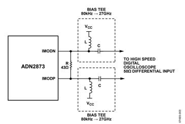
Figure 3. High Speed Electrical Test Differential Output Circuit
