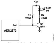
Figure 37. FAIL Indication Circuit
