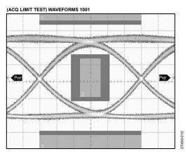
Figure 26. Optical Eye 2.488 Gbps, 65 ps/DIV, PRBS  $2^{31-1}$  $P_{AV} = 0 \text{ dBm}$ , ER = 9 dB, Mask Margin 22%, T<sub>A</sub> = 25°C
