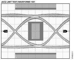
Figure 27. Optical Eye 2.488 Gbps, 65 ps/DIV, PRBS  $2^{31-1}$  $P_{AV} = -0.2$  dBm, ER = 8.96 dB, Mask Margin 21%,  $T_A = 85^{\circ}$ C
