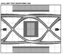
Figure 23. Optical Eye 2.488 Gbps, 65 ps/DIV, PRBS  $2^{31-1}$ P<sub>AV</sub> = -4.5 dBm, ER = 9 dB, Mask Margin 25%
