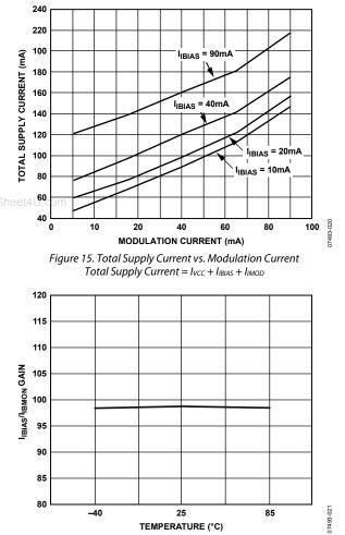
Figure 16. IIBIAS/IIBMON Gain vs. Temperature, IIBIAS = 11 mA
