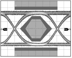
Figure 24. Optical Eye 622 Mbps, 264 ps/DIV, PRBS  $2^{31-1}$ P<sub>AV</sub> = -4.5 dBm, ER = 9 dB, Mask Margin 50%
