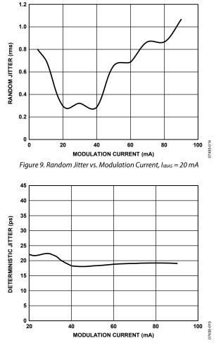
Figure 10. Deterministic Jitter at 2.488 Gbps vs. Modulation Current, I<sub>IBIAS</sub> = 20 mA
