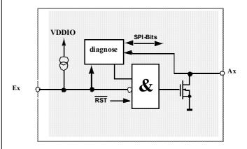
The transmit-function has to be enabled via SPI soft reset after an active RST (low). The open-drain outputs are current-limited, in addition the output voltage on Ax (x=1;2) is monitored for plausibility. If the voltage at Ax still exceeds a certain defined threshold after switch on the output transistor and after a predefined time tvoff, a short-circuit to battery is detected and the stage is turned off.
