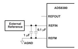
Figure 49. ADS8380 Using External Reference
