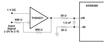
Figure 52. Bipolar Input Drive Configuration
