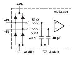
Figure 50. Simplified Analog Input
