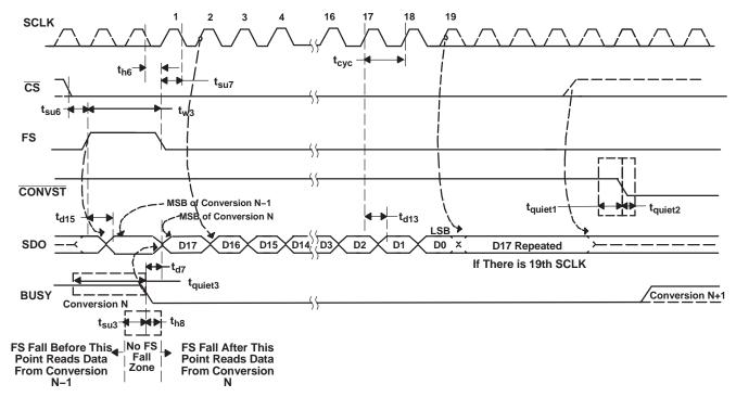
Figure 47. Read Frame Controlled via FS (FS is High When BUSY Falls)
