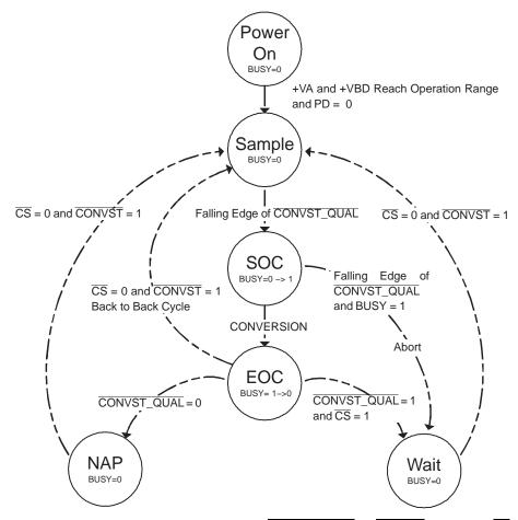
A. EOC = End of conversion, SOC = Start of conversion,  $\overline{\text{CONVST\_QUAL}}$  is  $\overline{\text{CONVST}}$  latched by  $\overline{\text{CS}}$  = 0, see Figure 39.
