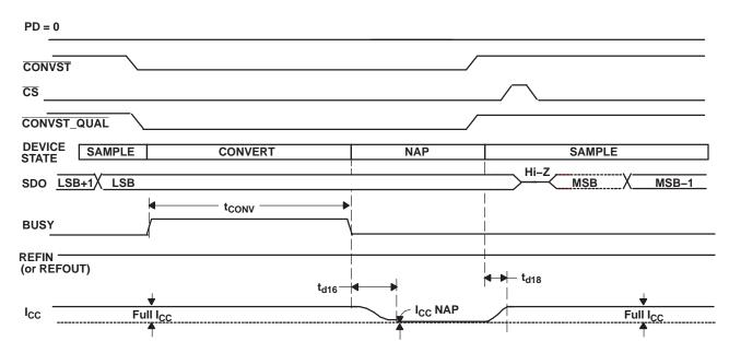
Figure 55. Device Nap Power Down/Resume
