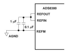
Figure 48. ADS8380 Using Internal Reference
