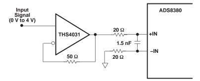
Figure 51. Unipolar Input Drive Configuration
