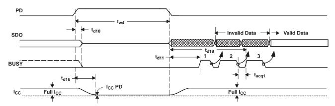
Figure 54. Device Full Power Down/Resume (External Reference Used)
