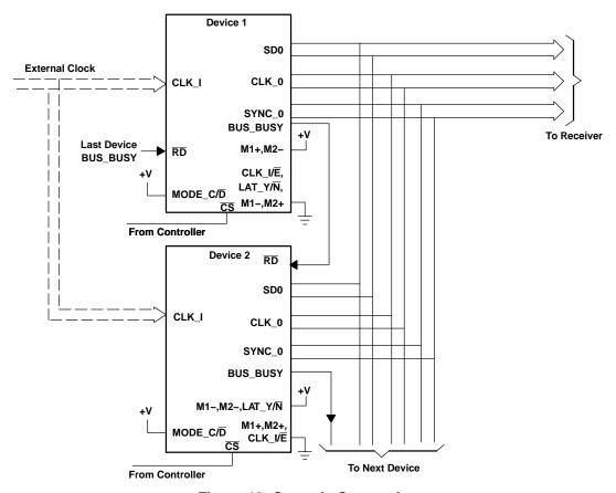
Figure 13. Cascade Connection
