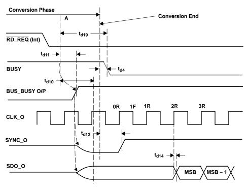
Figure 6. Start of Data Read Cycle with End of Conversion
