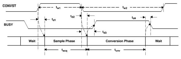
Figure 1. Sample and Convert With Wait (Less Than 2 MSPS Throughput)
