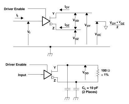
Figure 52. Driver Voltage and Current Definitions
