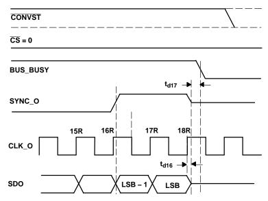
Figure 8. Data Read Cycle End with MODE  $C/\overline{D} = 1$
