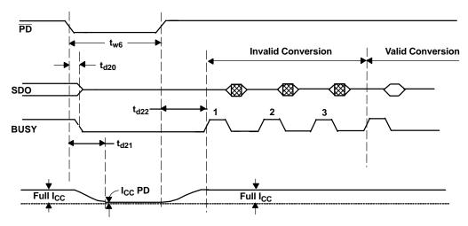
Figure 23. Device Full Powerdown and Powerup Sequence with Device Operation in External Reference Mode
