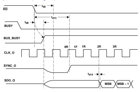
Figure 5. Start of Data Read Cycle with RD with CS Low and Device in Wait or Sample Phase
