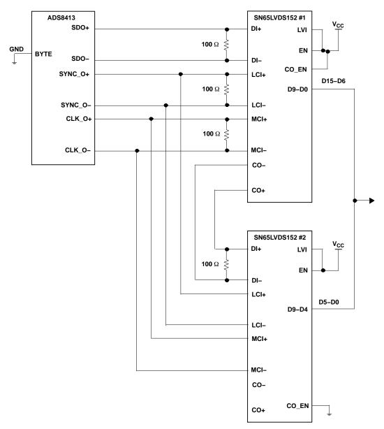
Figure 20. 16-Bit Data De-Serialization While BYTE = 0
