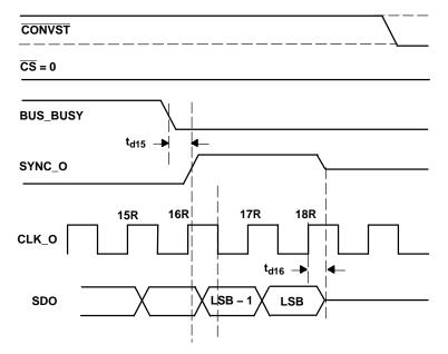
Figure 7. Data Read Cycle End with MODE  $C/\overline{D} = 0$
