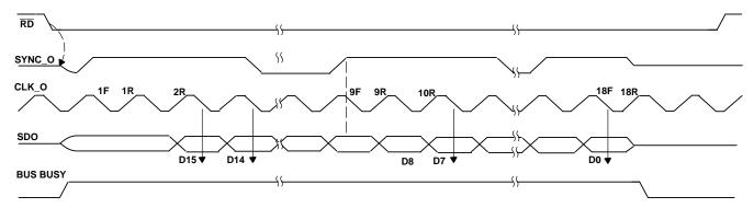
Figure 4. Data Read Timing Diagram with  $\overline{CS}$  Low and BYTE = 1
