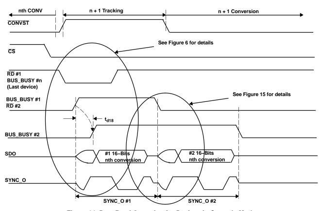
Figure 14. Data Read Operation for Devices in Cascade Mode
