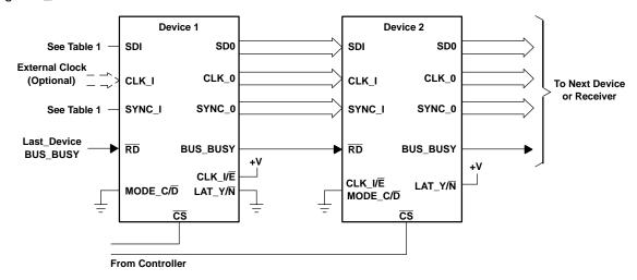
Figure 10. Connecting Multiple Devices in Daisy Chain
