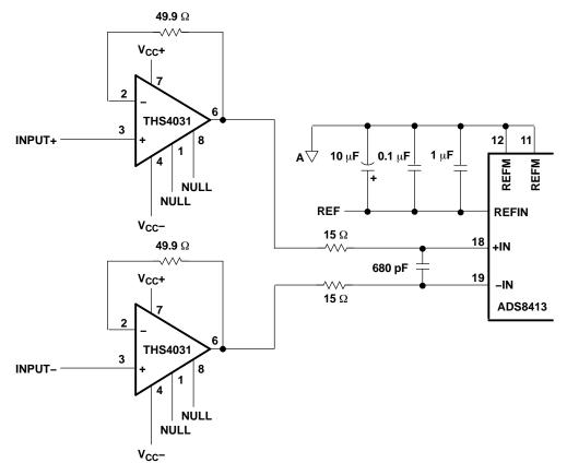
Figure 17. Typical Analog Input Schematic
