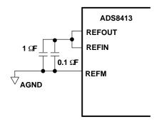
Figure 18. Using Internal Reference
