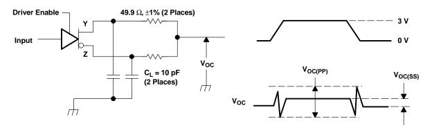
Figure 54. Test Circuit and Definitions for the Driver Common-Mode Output Voltage
