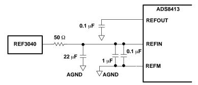
Figure 19. Using External Reference
