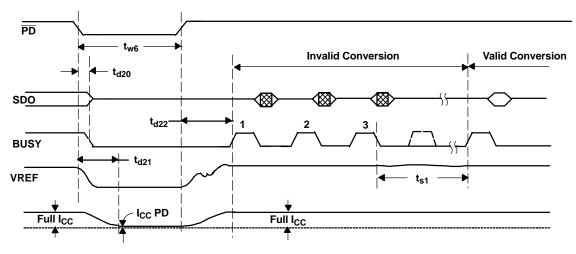
Figure 22. Device Full Powerdown and Powerup Sequence with Device Operation in Internal Reference Mode
