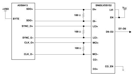
Figure 21. 8-Bit Data De-Serialization While BYTE = 1, Data
