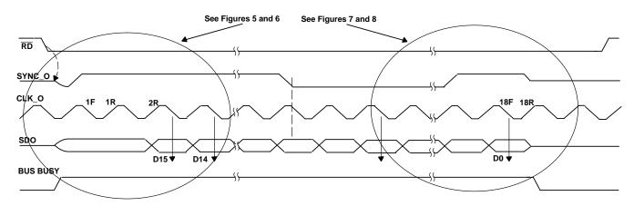
Figure 3. Data Read With  $\overline{CS}$  Low and BYTE = 0
