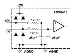
Figure 16. Simplified Input Circuit
