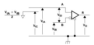
Figure 55. Receiver Voltage Definitions
