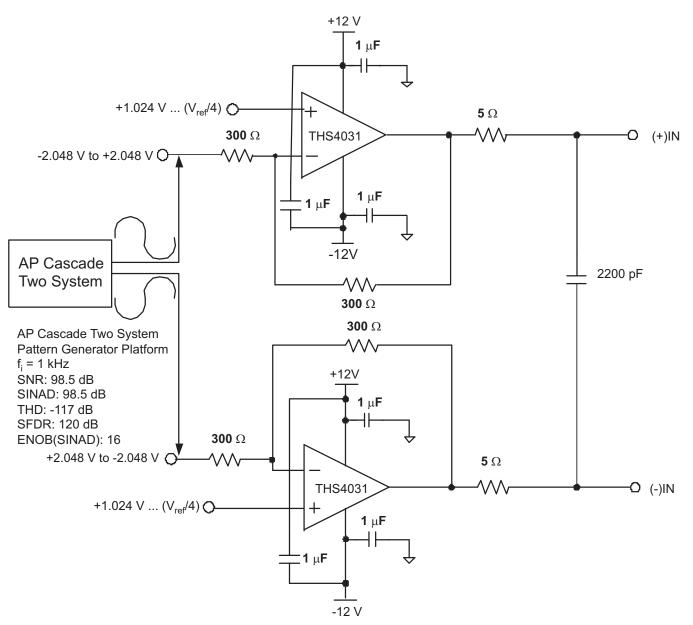
Figure 41. Differential Input, Differential Output Configuration
