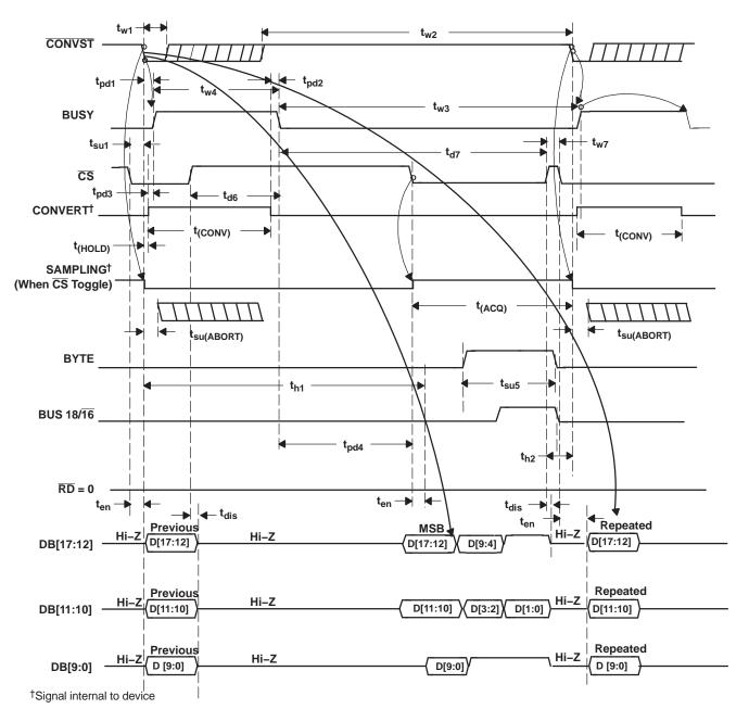
Figure 32. Timing for Conversion and Acquisition Cycles With CS Toggling, RD Tied to BDGND
