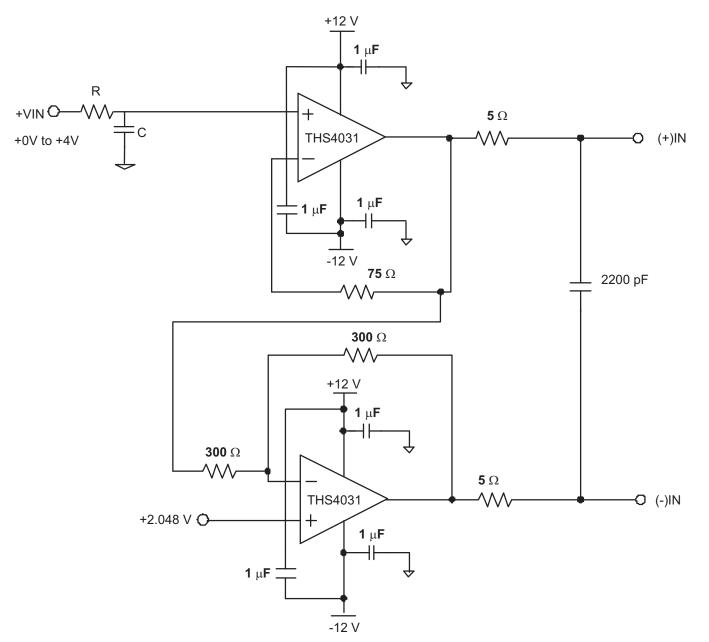
Figure 40. Single-Ended Input, Differential Output Configuration
