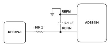
Figure 38. ADS8484 Using External Reference
