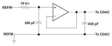
Figure 39. Simplified Reference Input Circuit
