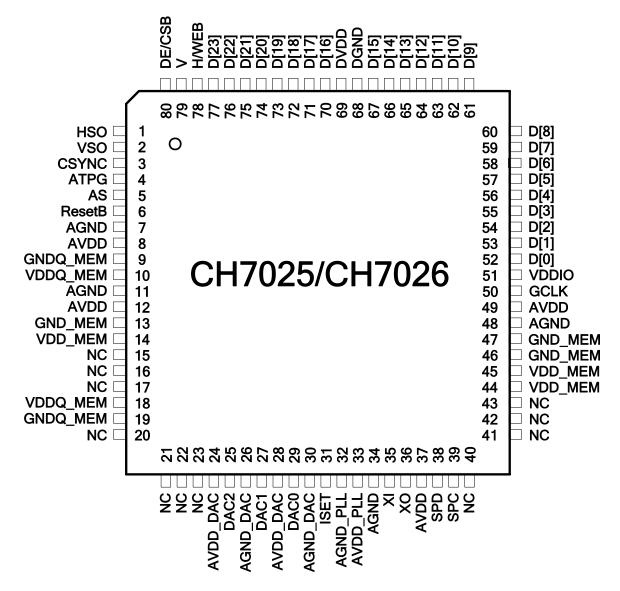
Figure 3: 80 Pin LQFP Package
