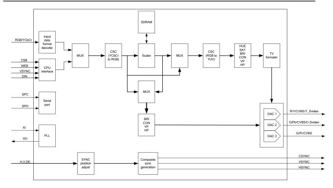
Figure 1: CH7025/CH7026 block diagram
