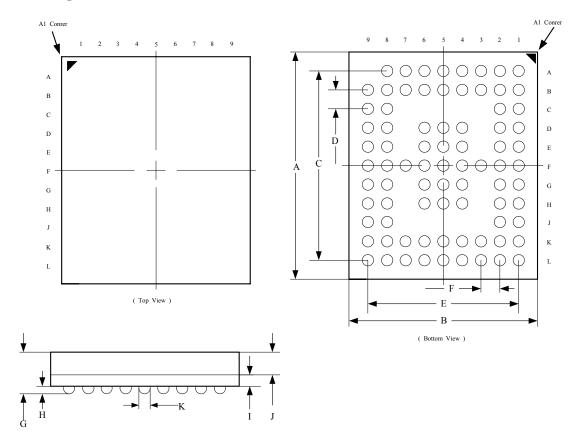
Figure 4: 80 Pin BGA Package
