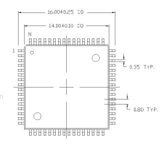
DIMENSIONS IN MILLIMETERS LEAD COPLANARITY 0.102 MAX.
