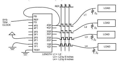
Figure 3. Programmable-Skew Clock Driver
