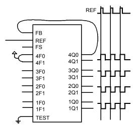
**Figure 4. Inverted Output Connections**
