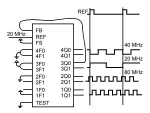
Figure 5. Frequency Multiplier with Skew Connections
