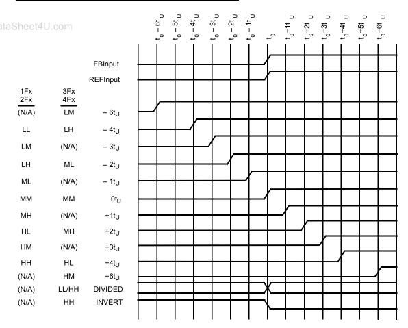
Figure 1. Typical Outputs with FB Connected to a Zero-Skew Output<sup>[3]</sup>
