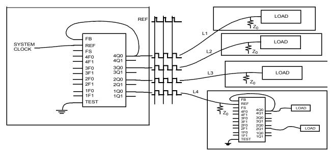
Figure 8. Board-to-Board Clock Distribution
