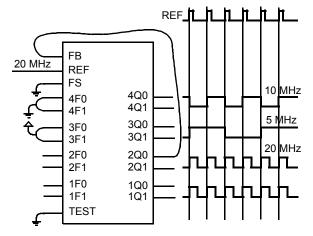
Figure 6. Frequency Divider Connections
