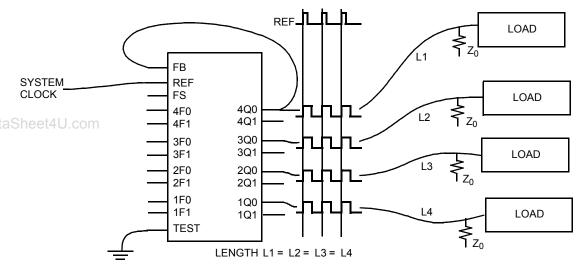
Figure 2. Zero-Skew and/or Zero-Delay Clock Driver
