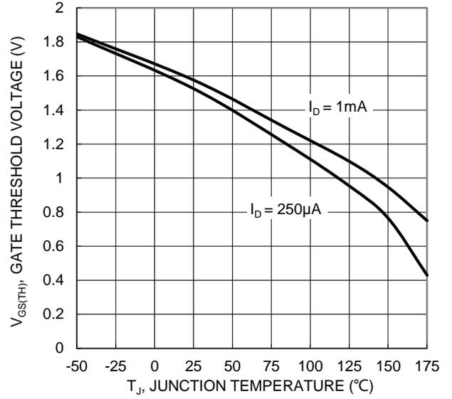
Figure 8. Gate Threshold Variation vs. Junction Temperature
