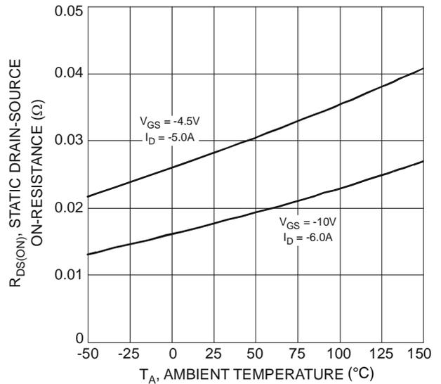
Fig. 4 Static Drain-Source On-Resistance vs. Ambient Temperature
