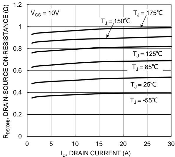
Figure 5. Typical On-Resistance vs. Drain Current and Temperature
