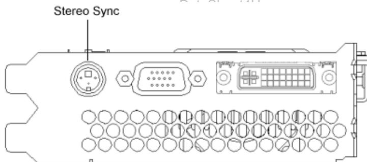
Figure 6. Stereo Output Port (Shown On Wildcat 4110)
