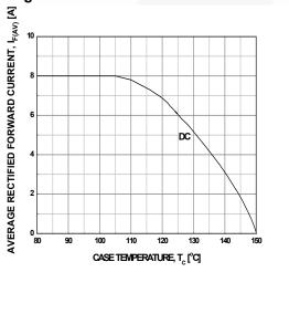
Figure 8. Forward Current Deration Curve
